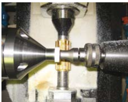
The acetal gears (three at a time) in readiness for gear cutting
