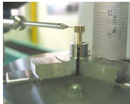
One of the small brass gears, all 4.8mm of it, being measured in our CNC gear measuring machine
